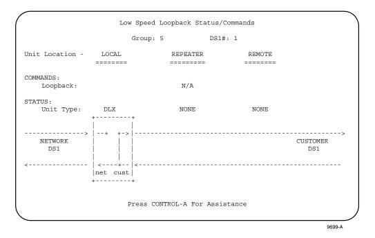
Figure 541-11a. DLX Customer Loopback Screen
